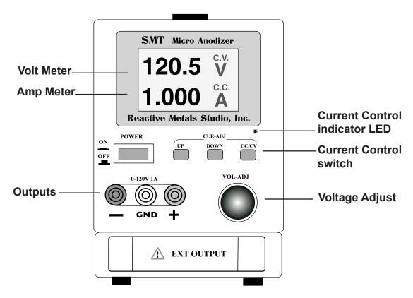
The built in **Multimeter** shows both **DC VOLTS** and **AMPERAGE**. The voltage is set and can be changed by turning the ten turn **VOLT-AGE ADJUST** knob. Voltage can be set accurately and will be indicated on the top row of numerals. The **AMPS/AMPERAGE** is set with the **UP/DOWN CURRENT ADJUST** buttons. Current output is shown in the bottom row of numerals.
