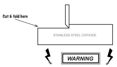
The alligator clips cannot be submerged in the electrolyte.
