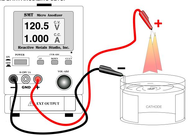
**VOLTAGE:** The **VOL-ADJ** knob is used to set voltage output, this in turn controls the color generated. It is a ten turn pot which allows for very accurate control. The voltage to endicate the voltage available prior to applying a load. The voltage can be adjusted at anytime. During anodizing the voltage will drop and then return as the color develops. Always turn the voltage **DOWN to Zero** when you turn the SMT **OFF**.
