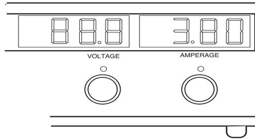
The **METER** array shows both volts and the amperage that is available. The voltage is set and can be changed by turning the ten turn **VOLTAGE** knob. Voltage can be set very accurately and will be indicated on the left. The voltage above is 88.8Vdc. The voltmeter indicates the voltage available prior to applying a load and can be adjusted at anytime. When the anodizing load is applied the voltage will drop and then rise as the process continues to the preset value.
