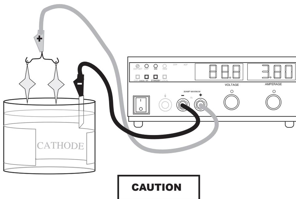
*The alligator clips can not be submerged in the electrolyte.*
